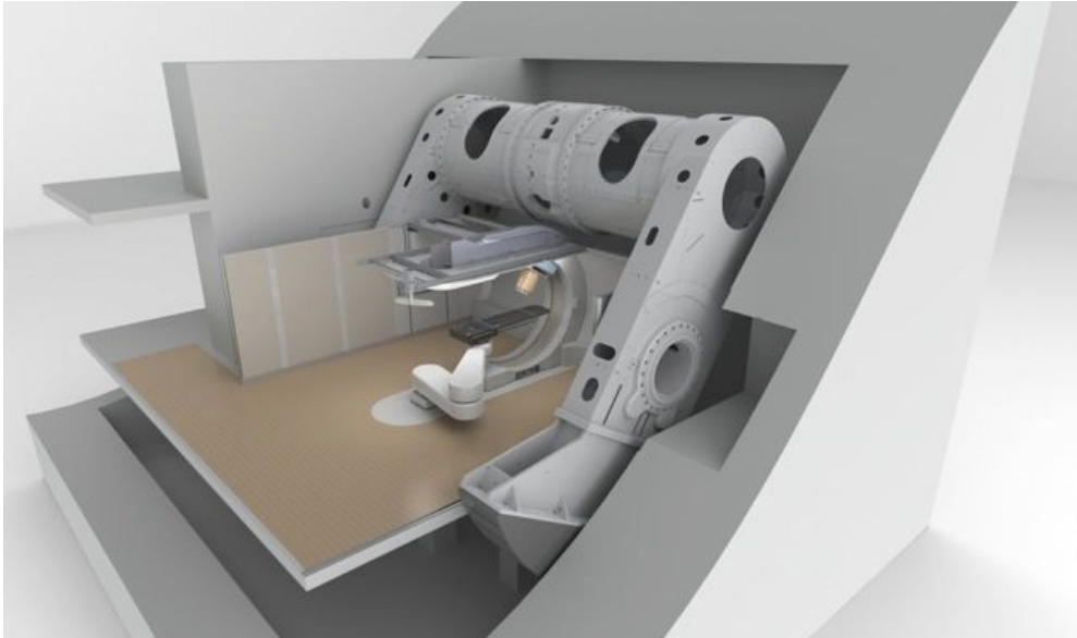
Figure 8. Behind the scenes view of the PBRT system. The patient positioning table coordinates with the proton beam to give a precise, image-guided exposure in full 3D. This is the most compact particle accelerator in the world.
