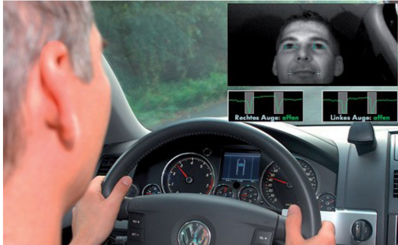
Figure 11. Volkswagen's driver assistance and integrated safety system uses Connex DDS to combine radars, laser range finders and video to assist safe operation. It tracks the driver's eyes to detect drowsiness. It also detects lane departures, avoids collisions and helps keep the car in its lane.
