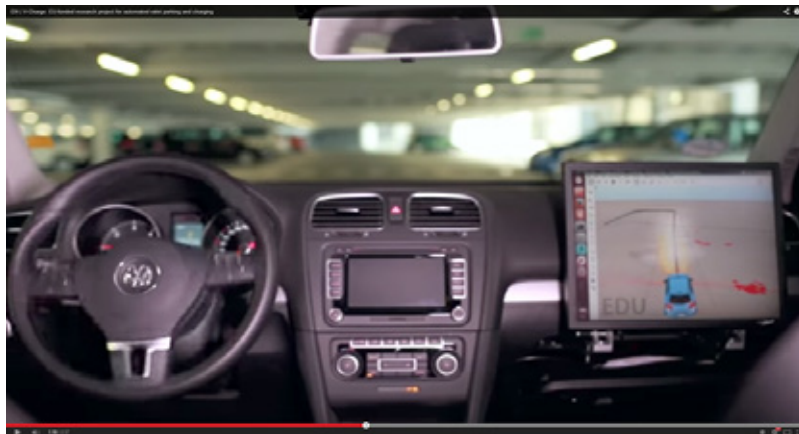
Figure 12. The V-Charge program, executed by VW, Bosch and ETH Zurich, implements an electric vehicle that can drop off its passenger, then drive autonomously to a parking lot, park itself and take its turn at a charging station. The system was successfully demonstrated in 2014.
