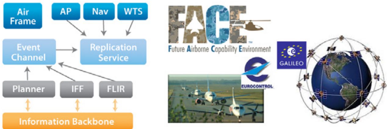
Figure 6. Modern, leading-edge CPS designs tend to be layered and componentized, standards and COTS-based, robust to failures, adaptive to operating conditions and cost effective to evolve and retarget.
