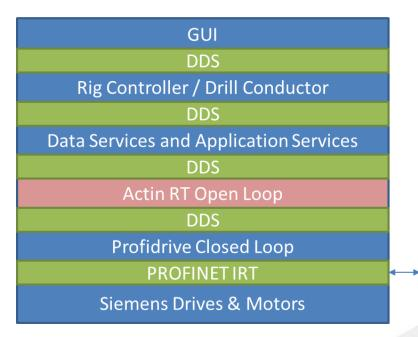
Powered by RTI DDS and Siemens Profinet real-time communication
