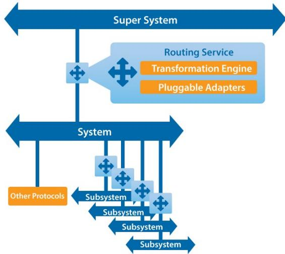
Figure 13. Routing Service chooses the correct information from each lower-level system and translates it into the “language” (data model) needed higher in the hierarchy. By also passing along QoS parameters, the entire system will look, at any one level, like a single logical data space. For a large system, that data space may hide a very complex actual topology. This abstraction enables large, integrated systems.
