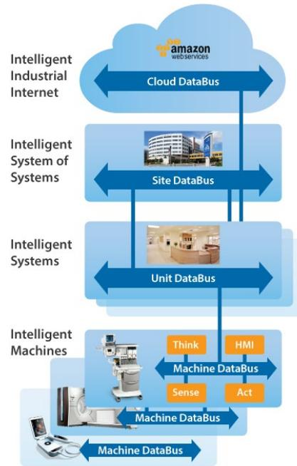
Figure 14. With routing and cloud technology integration, a DDS-based framework can integrate systems from deeply-embedded platforms all the way to cloud-based big data analytics.
