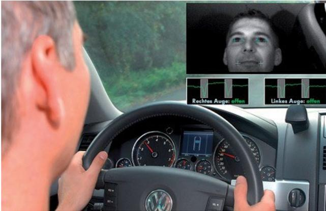
Figure 11. Volkswagen's driver assistance and integrated safety system uses Connex DDS to combine radars, laser range finders and video to assist safe operation. It tracks the driver's eyes to detect drowsiness. It also detects lane departures, avoids collisions and helps keep the car in its lane.
