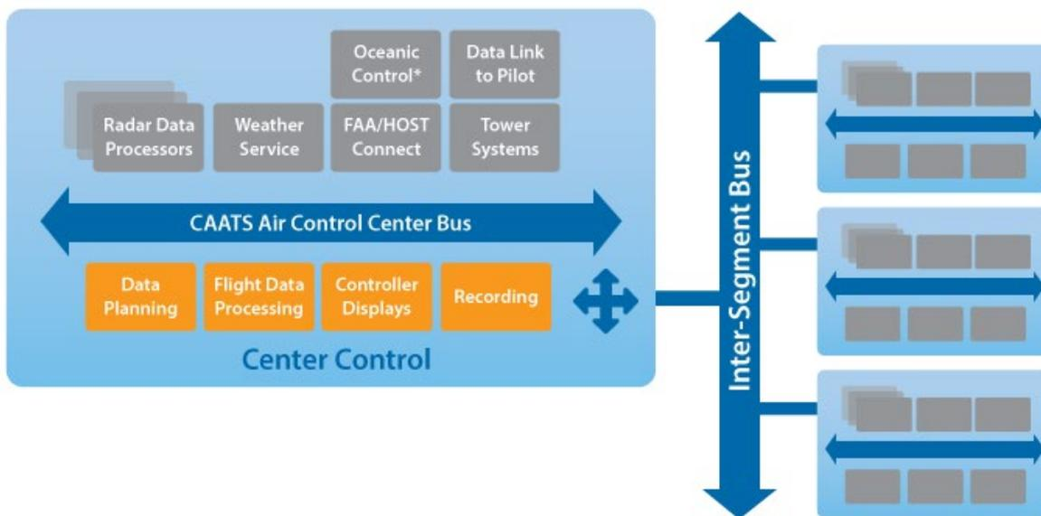
Figure 10. The CAATS integrates centers, communicates to external systems, and links segments together. Intra-center integration (green boxes) will be operational on RTI Connex DDS in 2015
