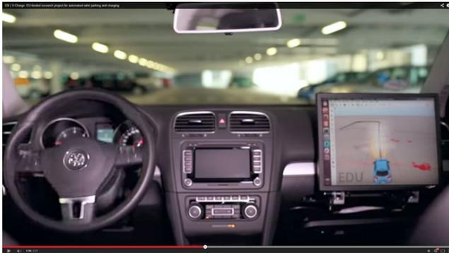
Figure 12. The V-Charge program, executed by VW, Bosch and ETH Zurich, implements an electric vehicle that can drop off its passenger, then drive autonomously to a parking lot, park itself and take its turn at a charging station. The system was successfully demonstrated in 2014.
