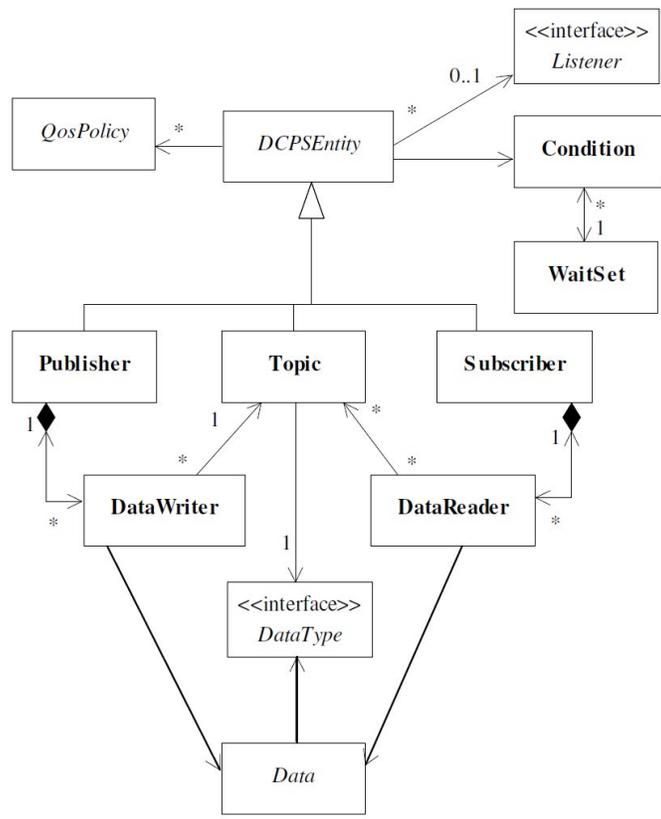
Figure 1. UML diagram of the DCPS model
