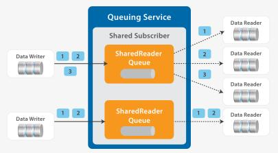
Each message is delivered to a single Data Reader in a round-robin manner. Based on the dispatch mode configured for a queue, Queuing Service will dispatch a message to a Data Reader that has explicitly indicated its availability, has acknowledged all its previous messages or is under a specified threshold of unacknowledged messages.
