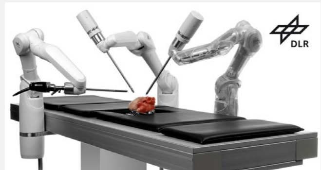
Figure 2. Three MiroLab robots coordinated through RTI Connex DDS software
